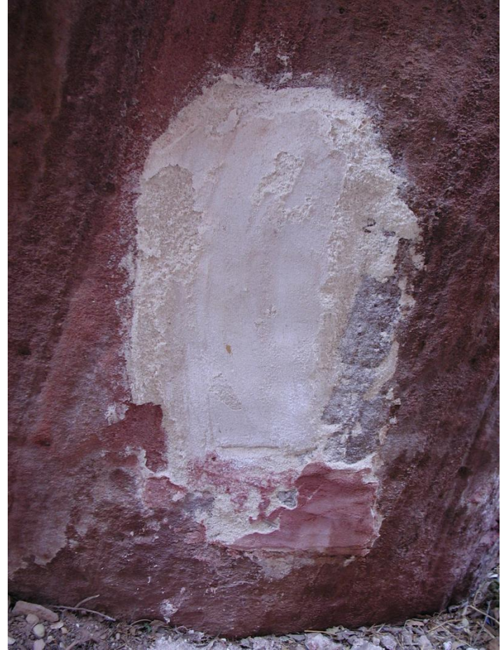
Sacrificed plaster ( Formula 6 ) applied on the freestanding sandstone block - material loss at the surface is recognizable.
